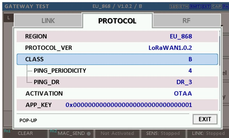
Fig 3.29 Selection of Class B in Parameter Configuration
