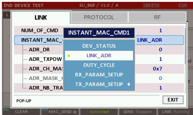
Fig 3.10 Example of a single MAC command selection
