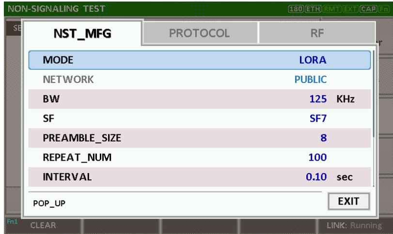
Fig 3.41 NST\_MFG Parameters for MFG Test (1/2)
