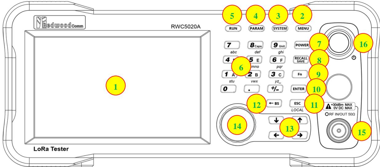
Fig 2.1 RWC5020A Front Panel View
