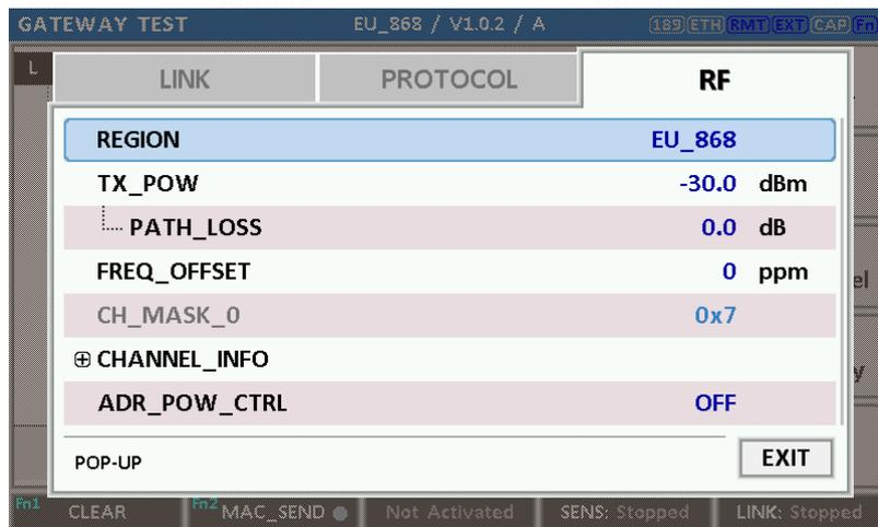
Fig 3.20 GWT Parameter Configuration Screen - RF
