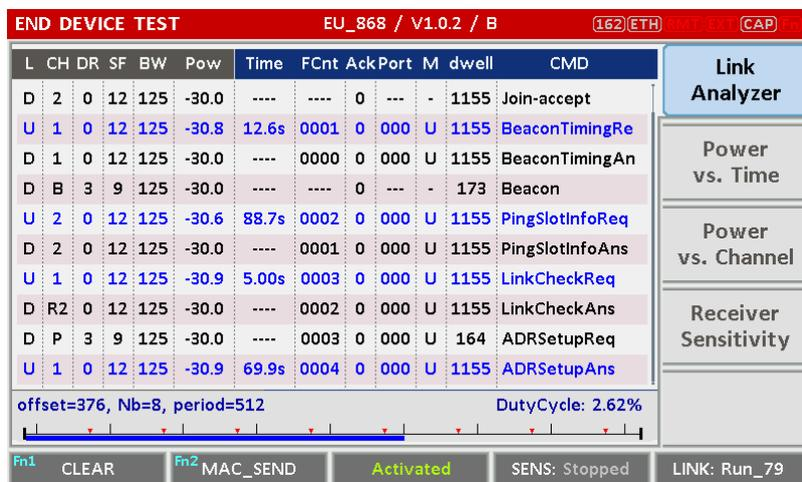
Fig 3.17 MAC command transmission through PING slot
