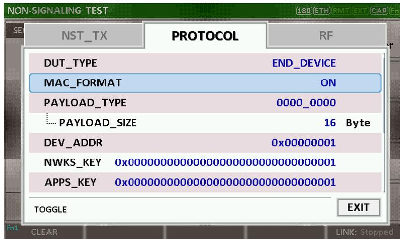
Fig 3.32 PROTOCOL Parameters 1/2 for Signal Generator
