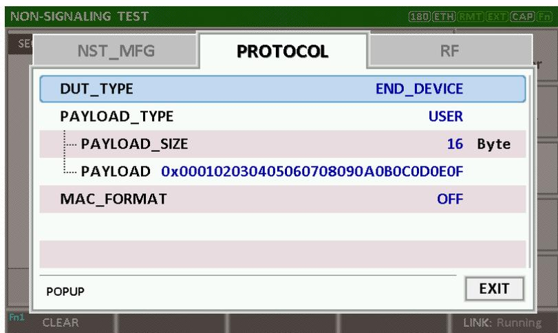
Fig 3.43 PROTOCOL Parameters for MFG Test
