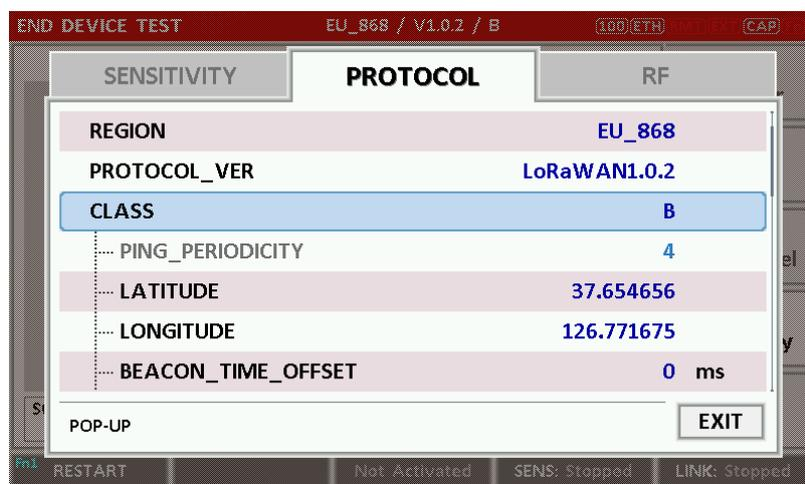
Fig 3.14 Selection of Class B in Parameter Configuration
