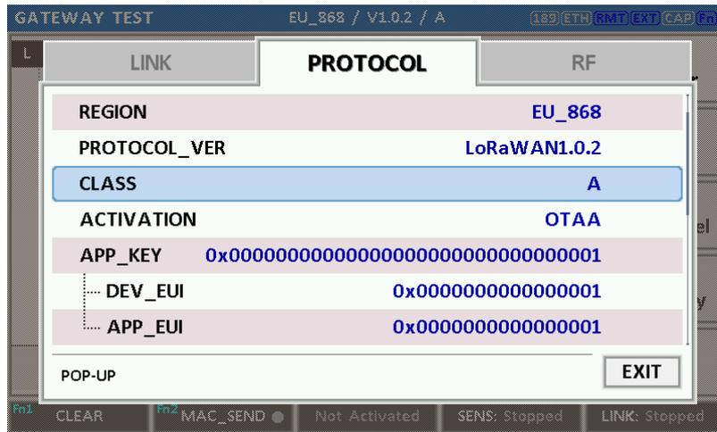
Fig 3.19 GWT Parameter Configuration Screen - PROTOCOL
