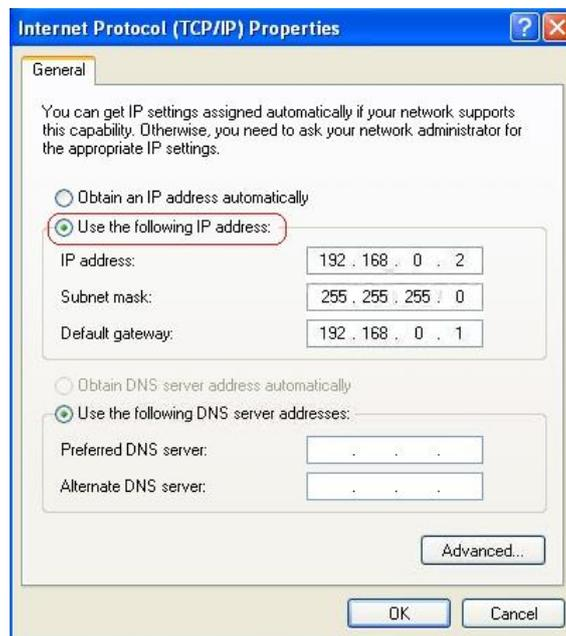
Fig 2.17 IP configuration of a remote PC
