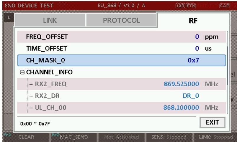
Fig 3.7 Channel Information in RF Parameters
